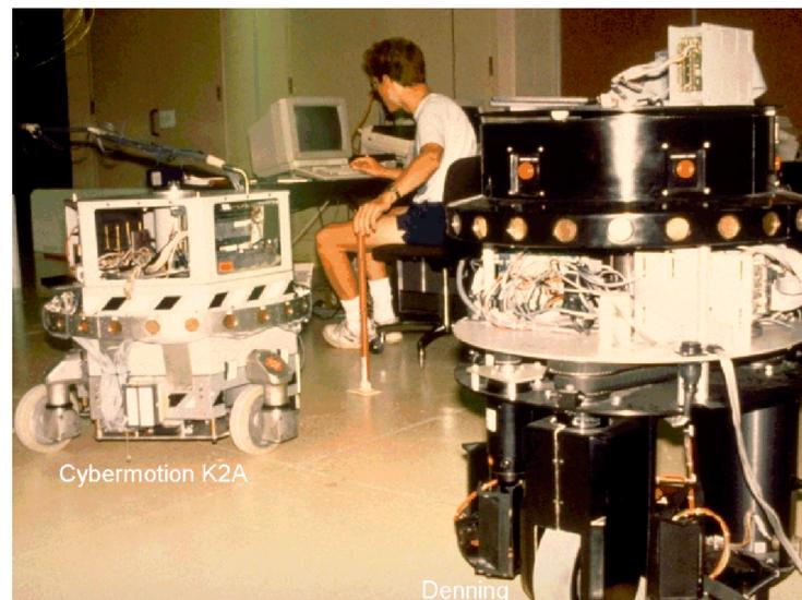
Figure 1.11: The Denning *Sentry* (foreground) incorporates a three-point *synchro-drive*
